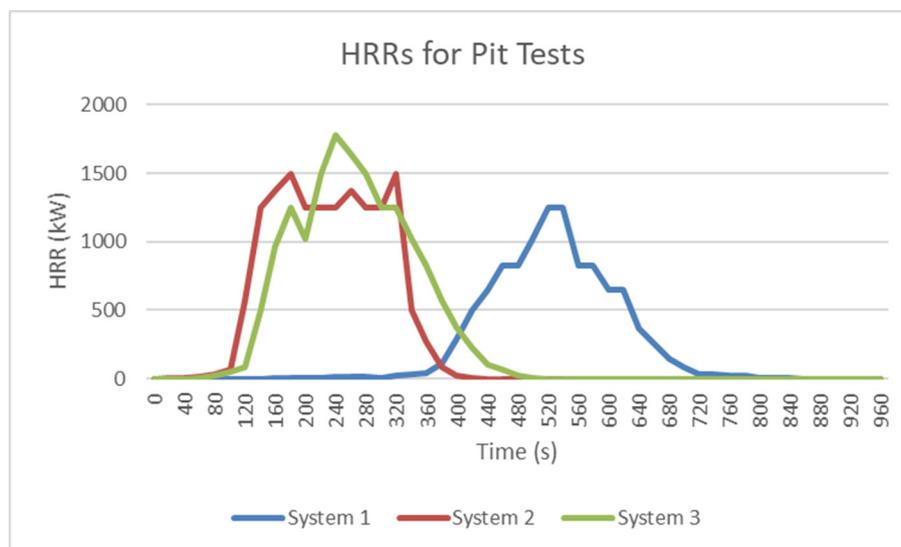
Fig. 1. Heat release rates (HRR) for the small scale pit test by System. System 1 contained flame retardants, System 2 was free of additive FR, and System 3 was free of additive FR and had a nylon cover. kW = kilowatt, s = seconds.
